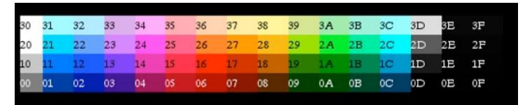
The palettes start at PPU address \$3F00 and \$3F10. To set this address, PPU port \$2006 is used. This port must be written twice, once for the high byte then for the low byte:
